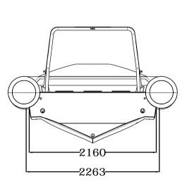
Length 863cm Beam 292cm 692cm Inside Length Inside Width 175cm 1040Kg Weight 24° Deadrise Max Pax 20/10 2000Kg Max Load 2\*200 Recommended HP Max HP 2\*250 XL Shaft Tube ф 56-40cm **Airtight Chambers**
